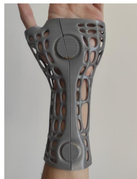
Fig.13. The finished prototype on the user's hand, locked using elastic bands wrapped around the circular elements
