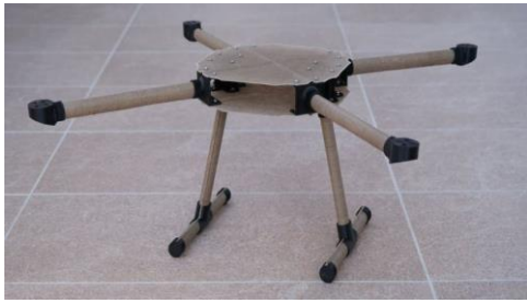
Fig.15. Drone frame made from biodegradable materials [19]
