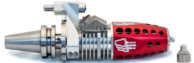
Fig.3. Laser DED extruder in a testing setup in a Haas VF series CNC machine [8]
