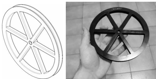
Fig.3. Geometrical model (left) and 3D printed sample (right) of the redirection pulley
