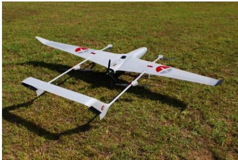
Fig.6. Carbonix Volanti: fixed wing carbon composite industrial drone with multirotor VTOL capability [7]
