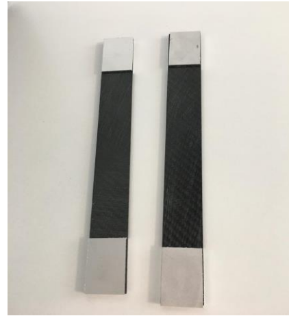
Fig. 4. CFRP samples prepared for tensile testing
