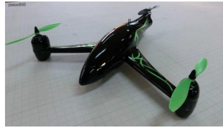
Fig.12. Tricopter made from fiberglass frame [16]
