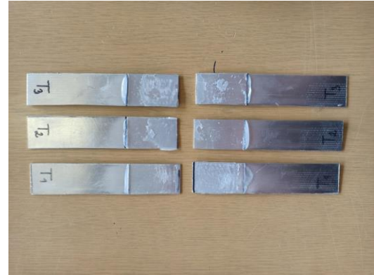
Fig. 9. Display of T samples after fracture
