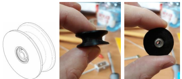
Fig.6. Geometrical model and fabricated sample of wheels
