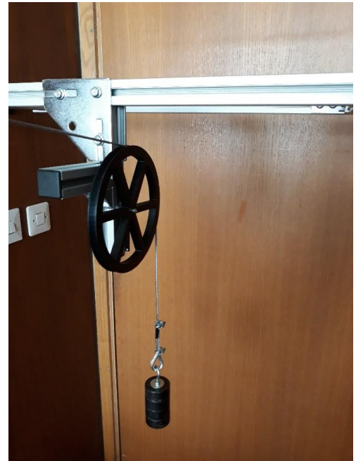
Fig.4. Redirection pulley mounted to the lower station
