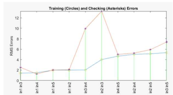
Fig.4. All two predictors combinations influence on the mean ablation depth of the excimer laser micromachining
