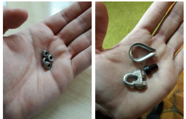
Fig.5. Bearings for redirection pulley and trolley wheel (left) and rope fastener clamp and thimble (right)
