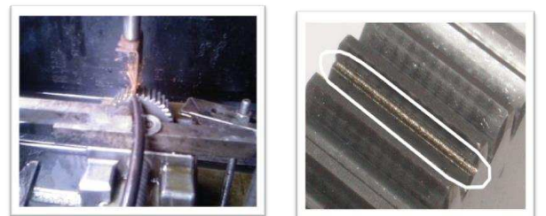
Fig.2 Damage gear tooth
