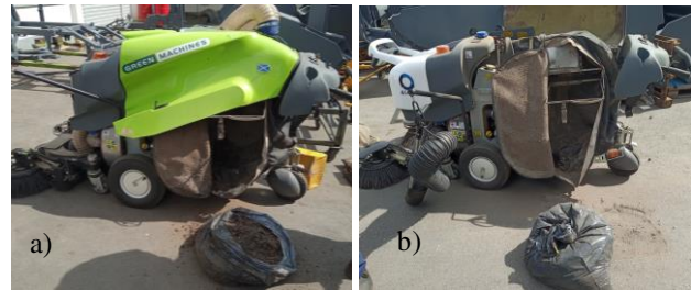
Fig.12. Sweepers: a) novel design with air-recirculation system and b) old sweeper with diesel engine
