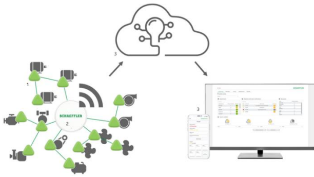
Fig.4. Basic components of "Optime" device [15]: 1- sensors, 2- Gateway (receiver / transmitter); 3- digital service
